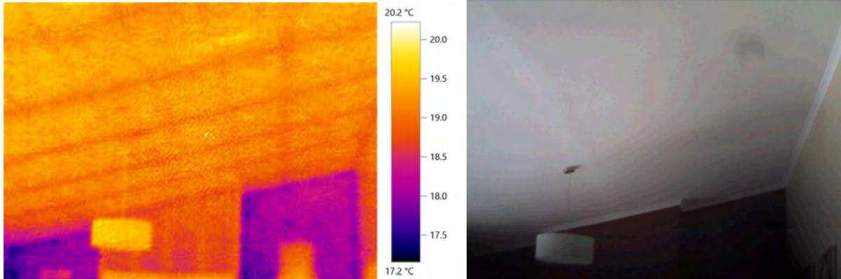
21. Thermography of kitchen A/C: seems dry enough underneath. Possible slight damp patch low down / at the noggings. Often an occasional overflow in humid weather, and/or the condensate pipe is leaking / blocked.
